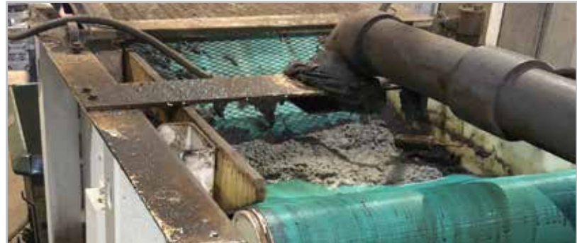
Continuous Loop Filter Belt - No Media Required
